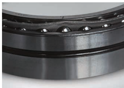
Part: Cage of an angular contact ball bearing Observation: Pressed-steel cage deformation Cause: Shock load due to poor handling
