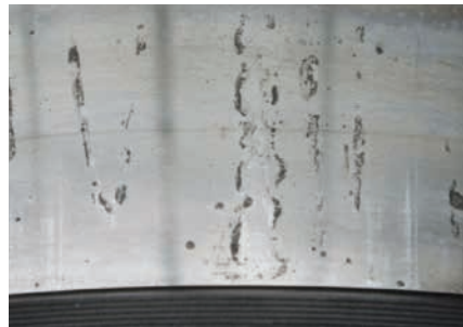
Part: Inner ring of a spherical roller bearing Observation: Rust on raceway surface at roller pitch Cause: Entry of water into lubricant
