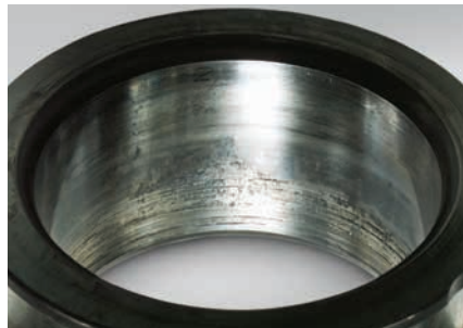
Part: Inner ring of a spherical roller bearing Observation: Creep accompanied by scoring of bore surface Cause: Insufficient interference
