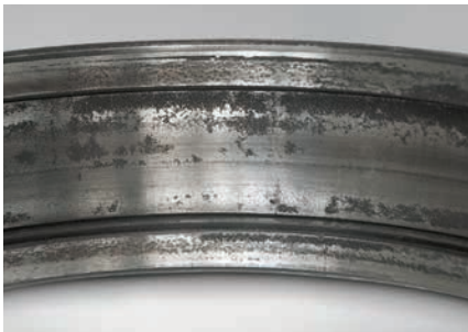
Part: Outer ring of a cylindrical roller bearing Observation: Rust on the rib face and raceway surface Cause: Poor lubrication due to water entry
