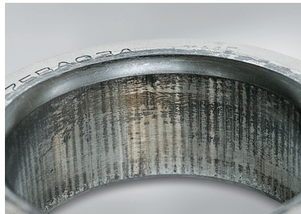
Part: Inner ring of an angular contact ball bearing Observation: Notable fretting occurs over entire circumference of bore surface Cause: Insufficient interference fit
