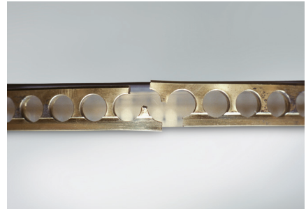
Part: Cage of an angular contact ball bearing Observation: Fracture of machined high-tension brass cage
