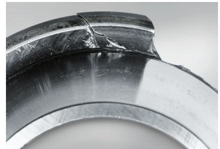
Part: Inner ring of a spherical thrust roller bearing Observation: Fracture occurs at the large rib Cause: Repeated load
