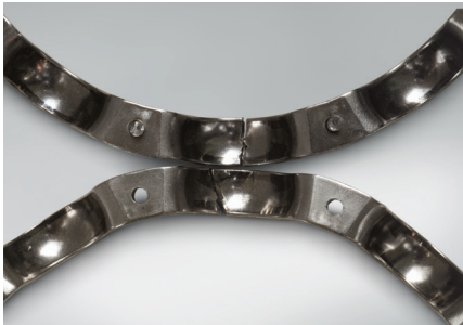
Part: Cage of a deep groove ball bearing Observation: Fracture of pressed-steel cage-pocket
