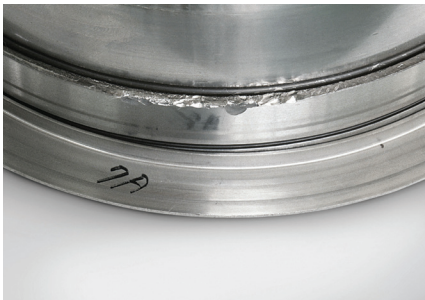
Part: Inner ring of a double-row cylindrical roller bearing Observation: Chipping occurs at the center rib Cause: Excessive load during mounting
