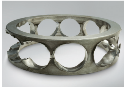
Part: Cage of an angular contact ball bearing Observation: Pocket pillar fractures from a cast iron machined cage Cause: Abnormal load action on cage due to misaligned mounting between inner and outer rings
