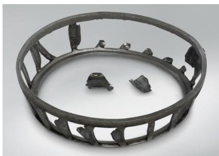
Part: Cage of a tapered roller bearing Observation: Pillar fractures of pressed-steel cage
