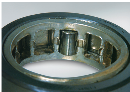
Part: Cage of a cylindrical roller bearing Observation: Deformation and wear of a machined high-tension brass cage
