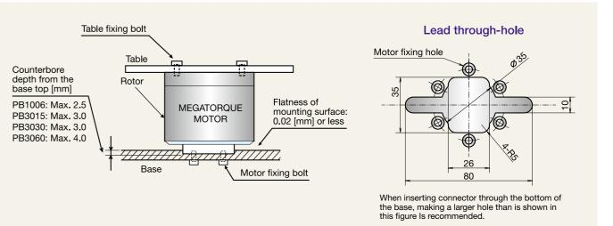
(Note) Since the installation condition shown below can cause mechanical resonant vibration or failure of estimation of magnetic pole due to low rigidity of the mounting base and the load, installation of motor to mounting base and load to motor have to be secure and rigid.
