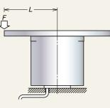
1) When F is an external force: • Axial load:  $F_a = F$  + total weight of jigs and works • Moment load: M = 0
