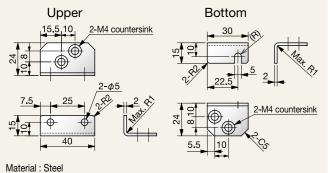
Surface treatment : Trivalent chrome coating Four screw bolts are attached.
