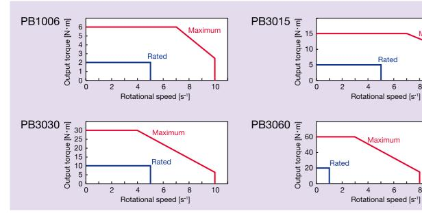
\*Speed - Torque curve is typical value measured in 200 [VAC] (PB3060 : 220 [VAC]).
